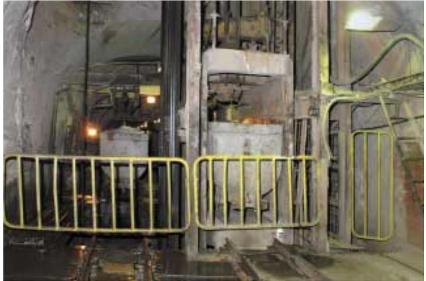
*Rail cars containing ore are currently hoisted in the shaft cages. This is of course a very labour intensive haulage and hoisting system with evident capacity deficiencies.*
