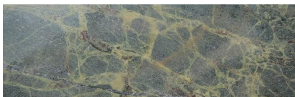
Calc-silicate altered basalt YDD0305 107m 0.90 g/t chlorite clinozoisite
