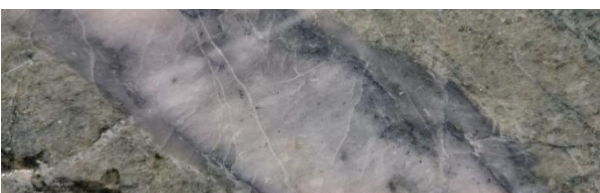
YDD0455 quartz molybdenite vein in altered granodiorite
