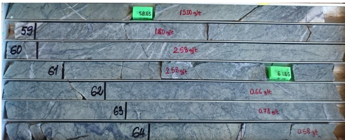
Figure 7-23 S1 Structure YDD0183 18m at 2.85 g/t
