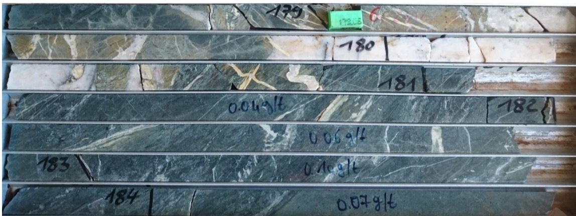
Figure 7-21 Y2 Structure YDD0184 6m at 5.53 g/t
