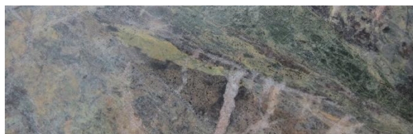
Calc Silicate altered basalt YDD0305 0.51 g/t garnet, epidote magnetite
