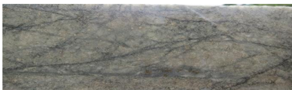
YDD0193 210m 5.14 g/t grey quartz chlorite tourmaline veined granodiorite
