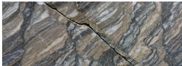
YDD0309 122m at 11.70 g/t Albite ankerite tourmaline altered basalt
