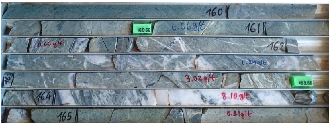
Figure 7-22 Y3 Structure YDD0335 18m at 2.85 g/t
