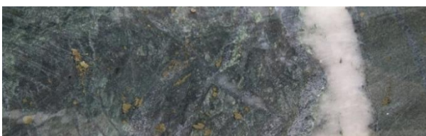
YDD0204 100m 0.80 g/t quartz carbonate veined pyrite altered basalt
