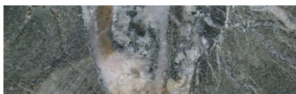
YDD0182 69m 2.00 g/t quartz carbonate veined chlorite altered basalt
