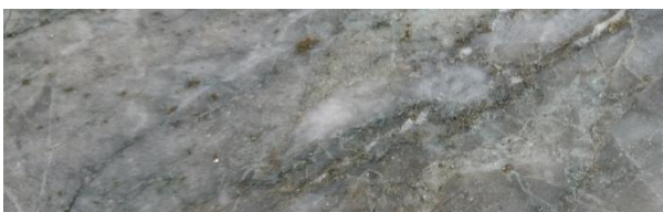
YDD0444 59m 19.00 g/t tourmaline muscovite chlorite pyrite grey quartz altered granodiorite
