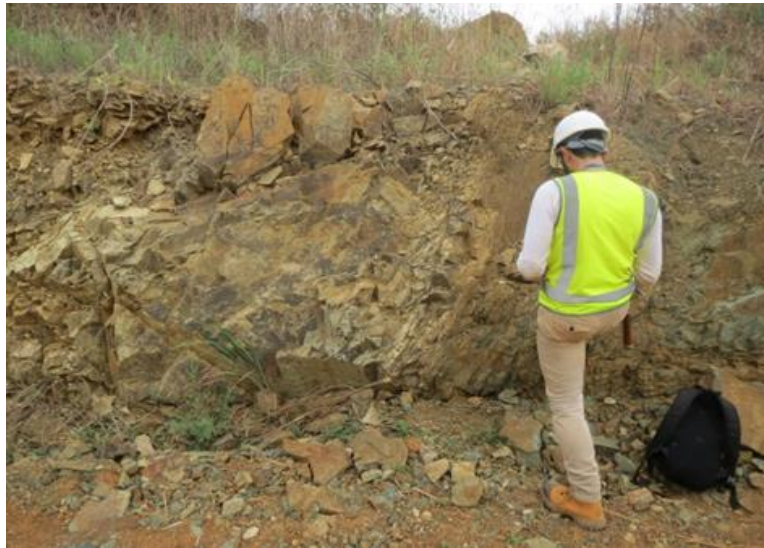
Figure 7-14 S2 Structure contact between basalt and quartz porphyry
