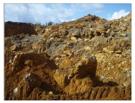
Figure 4-15: Irregular Pit Floor Showing Boulders (Photo Golder)
