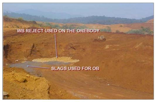
Figure 4-20: Use of Waste Material and Slag on Pit Floor (Photo PTI)
