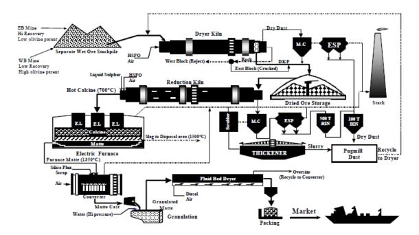
Figure 4-4: Process Flow Sheet for the PT Inco Plant (from Kroll et al, 2009b)
