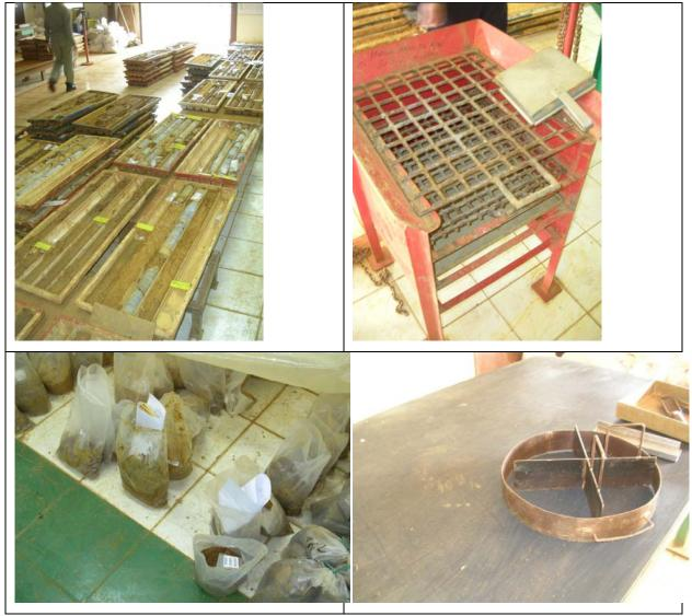
Figure 4-7: Core sample preparation
