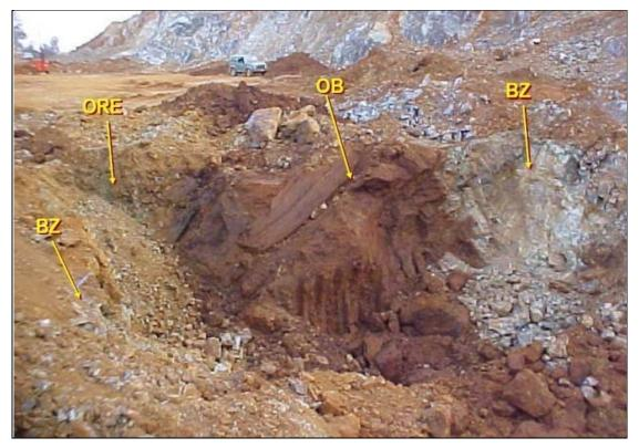
Figure 4-23: Ore Identification (Photo PTI)
