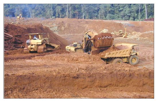
Figure 4-22: Overburden Stripping to Expose Ore (Photo PTI)
