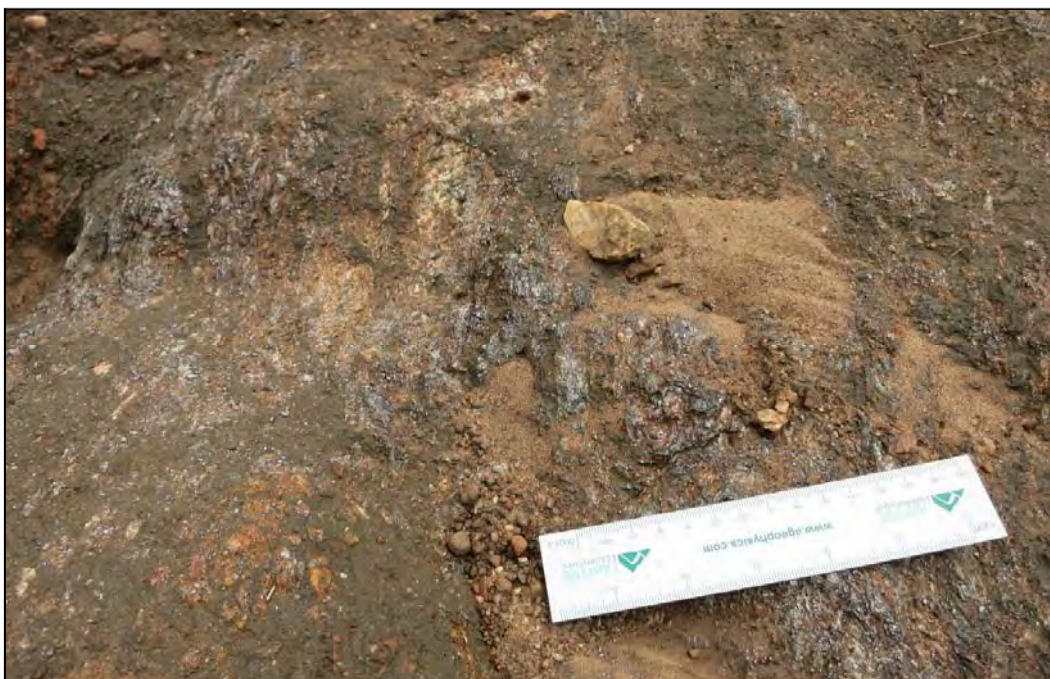
Figure 12. 7: Surface material with high graphite tenor (Photo J. Laforest 2013).
