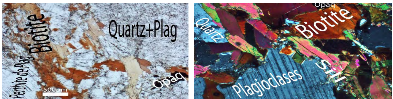
Figure 7. 2: Mineralogical assemblage of the paragneiss : Biot-Qtz-Pl-Fk-Opx-Fluides+ou-Mus-pyrite-rutile.
