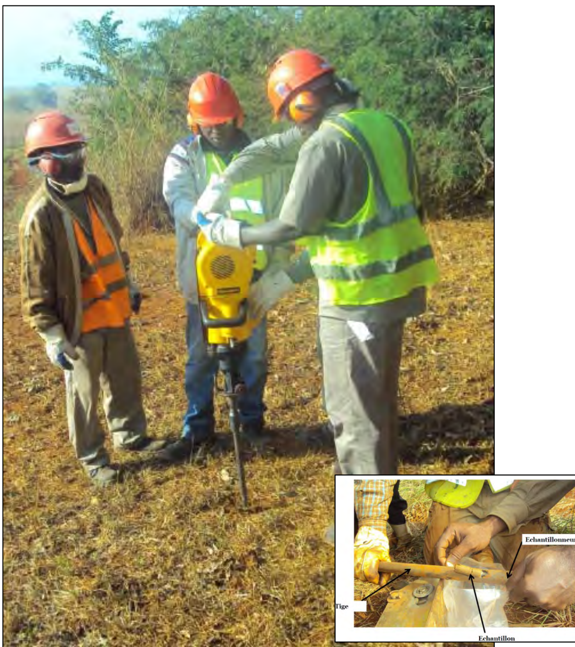
Figure 10. 1: Sampling using the Pionjar
