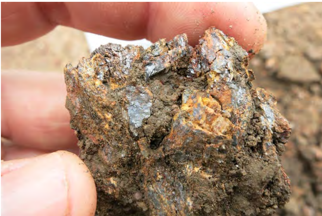
Figure 12. 6: Surface sample with high graphite tenor (Photo J. Laforest 2013).
