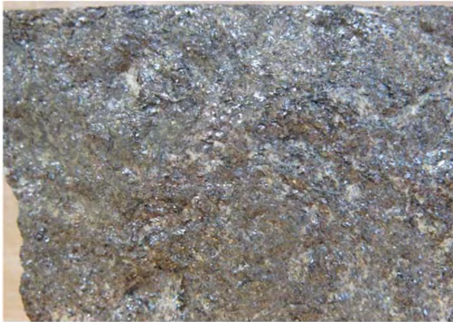
Figure 7. 7: Core photograph of the non-weathered paragneiss showing the graphite content.
