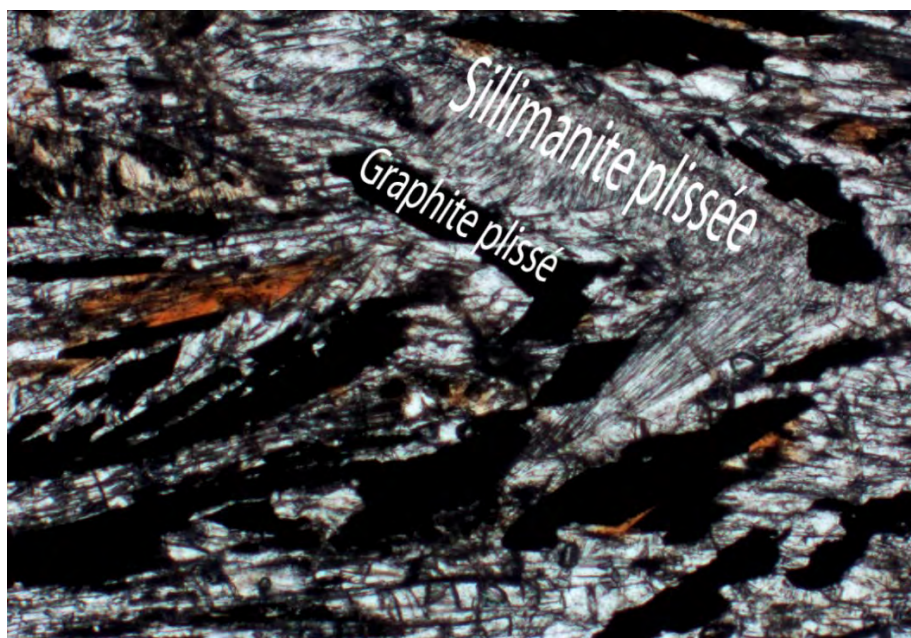
Figure 7. 6: Thin section showing graphite and sillimanite affected by the later tectonic event.
