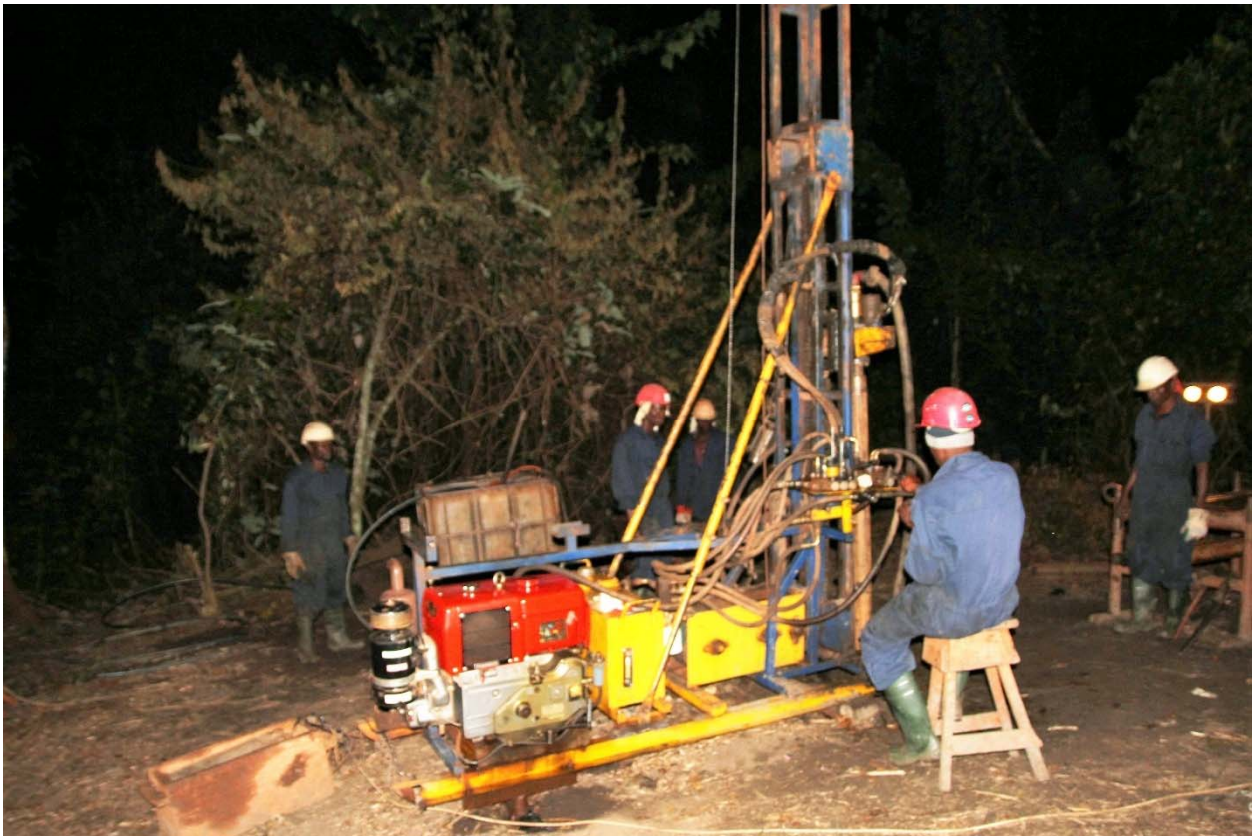
Figure 10. 3: Jacro diamond drilling rig in operation at the Lola Graphite (October 2013).
