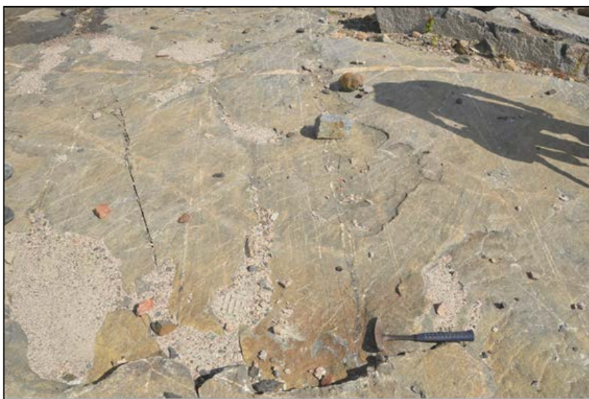
Figure 7.12 Exposed Mineralized Shear Zone in the South Pit
