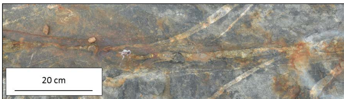
Figure 7.7 Mylonitic Shear with Quartz-Sulphide Vein (center) and Deformed Pre-mineral Bucky Quartz Veins Displaying Fault Drag. South Pit
