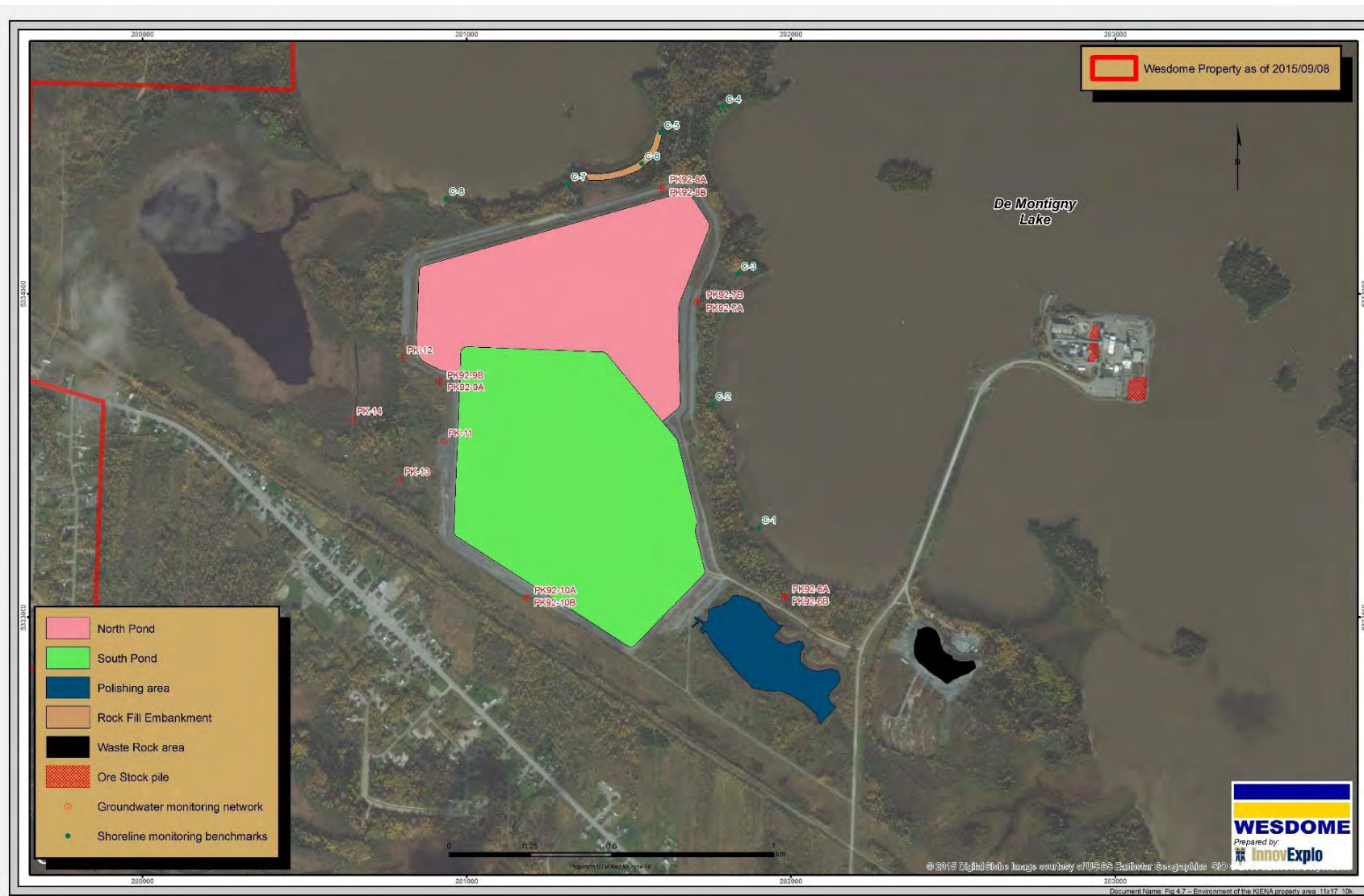
Figure 4.7 – Kiena mine site showing surface infrastructure, tailings deposition, and polishing pond.
