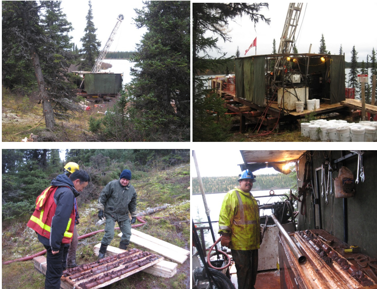
Figure 10-5: Downing Diamond Drills in Action during QP Site Visit Autumn 2013, Fresh Core Review from Both Drills
