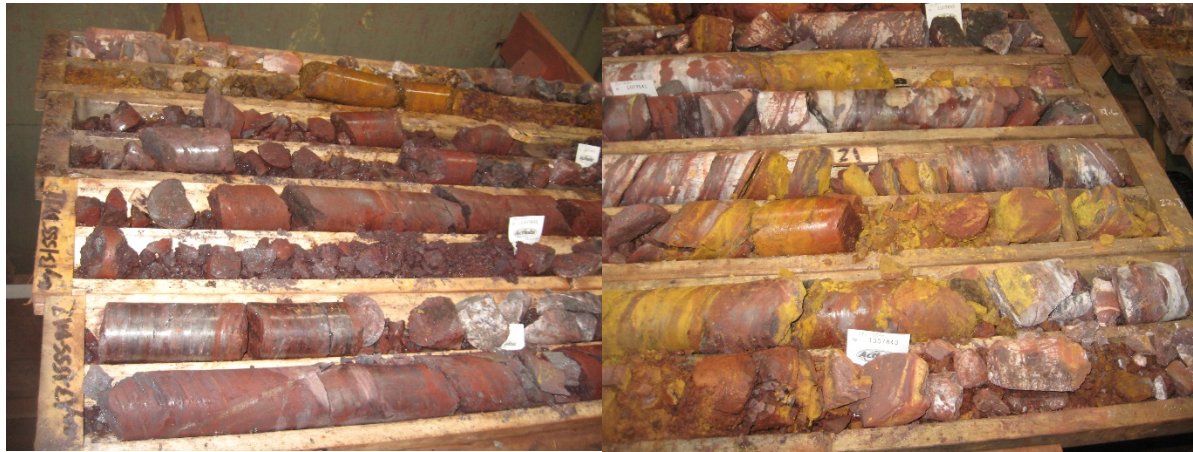
Figure 7-7: Mineralization of Red and Yellow DSO in Fresh Core
