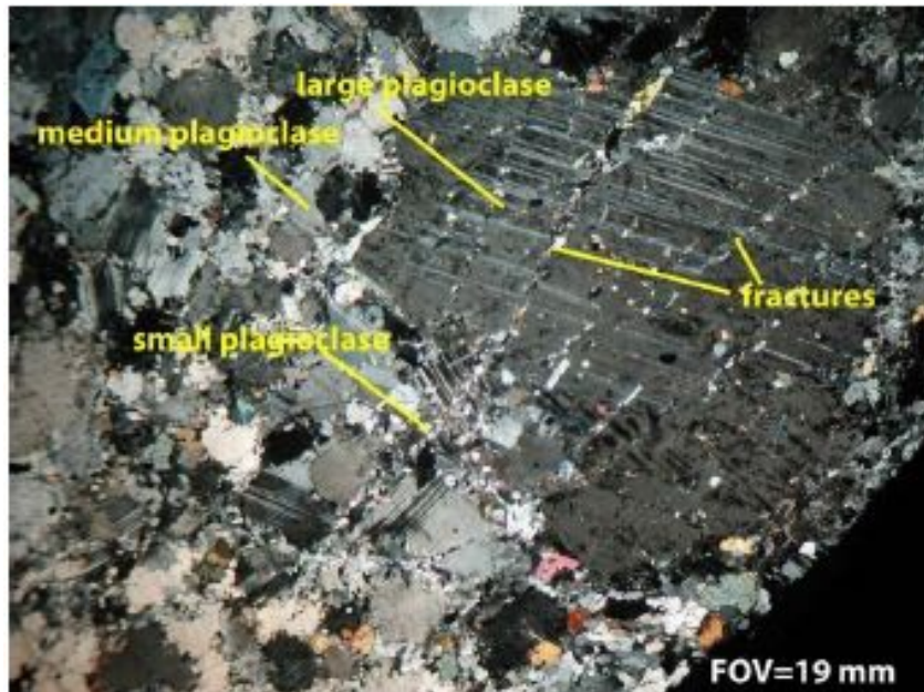
Figure 7-7 Micrograph showing three sizes of plagioclase
