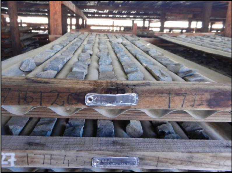
Photograph 4: View of the RTZ core – split for assay and well preserved in wood & metal core trays.
