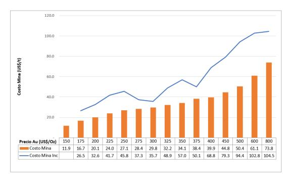
FIGURE 15-4 INCREMENTAL OPEN PIT MINING COST
