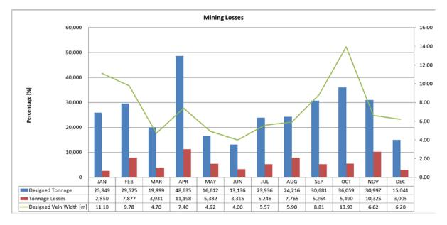
FIGURE 15-3 2016 MINING LOSSES AT GUANACO (CACHINALITO)
