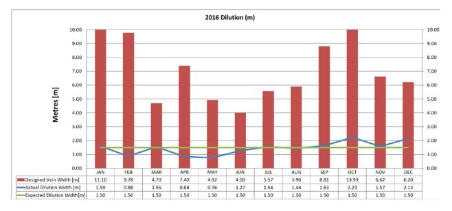
FIGURE 15-2 2016 DILUTION BY VOLUME AT GUANACO (CACHINALITO)
