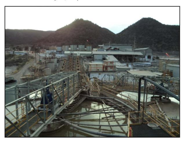
Figure 17-1 View of Leach Tanks and CCD Circuits
