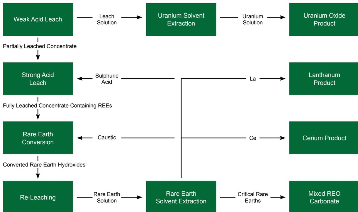
Figure 7. Metallurgical design of the refinery circuit.
