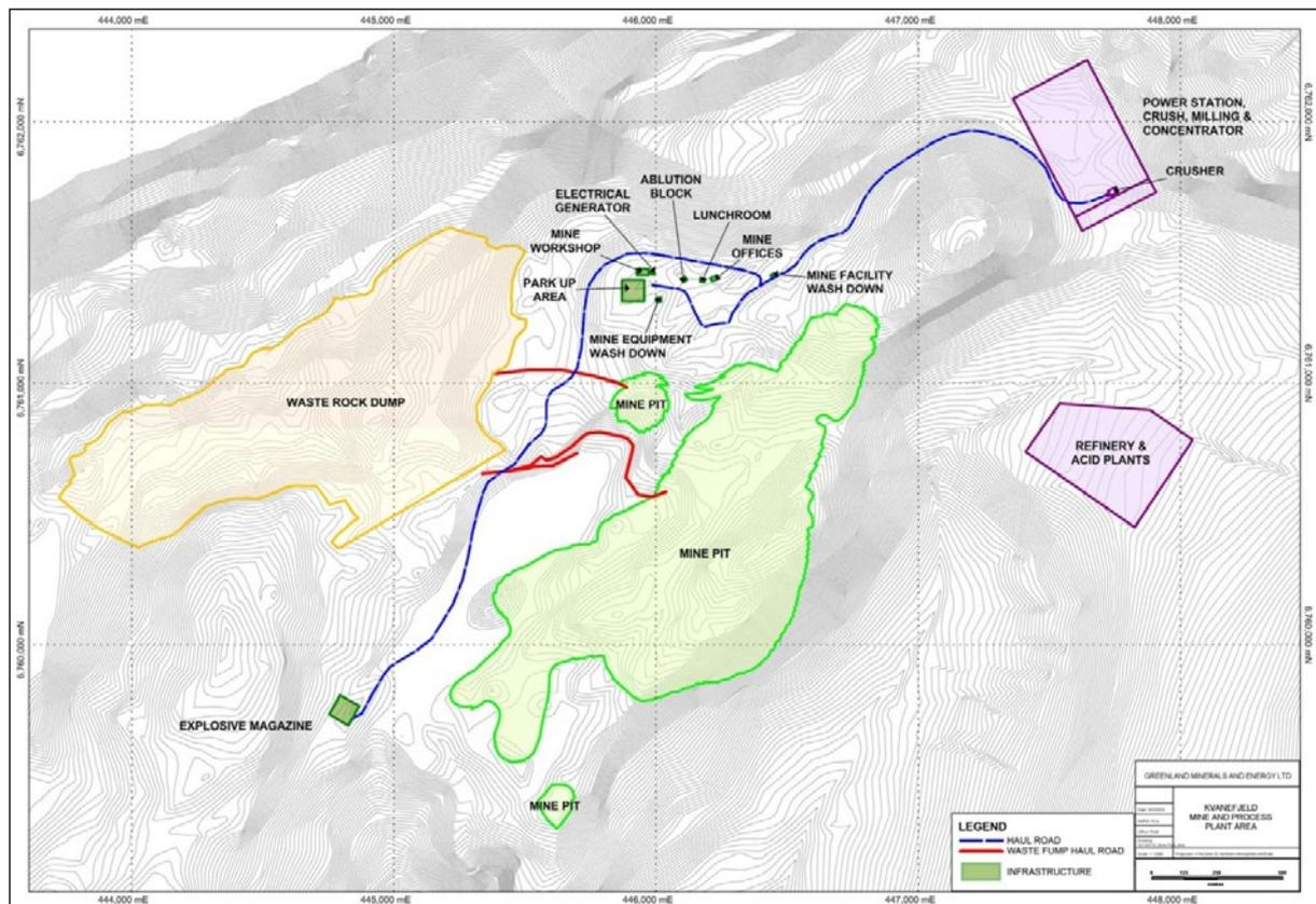
Figure 4. Plan of the Kvanefjeld area displaying the mine pit limits and facilities layout.
