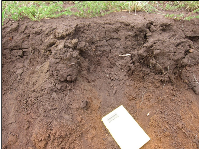
Figure 7.8: High slimes CL on low slimes CS_L material
