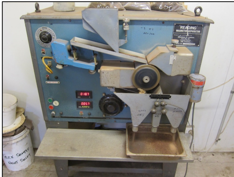
Figure 11.5: Current on site laboratory-based magnetic separator
