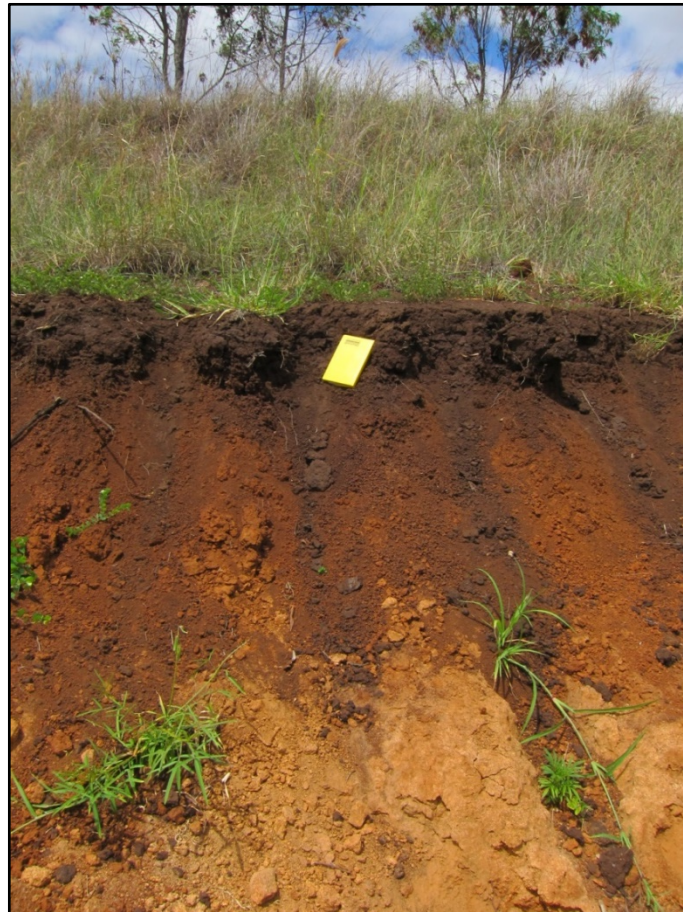
Figure 7.5: CS_H material sitting on DG Material
