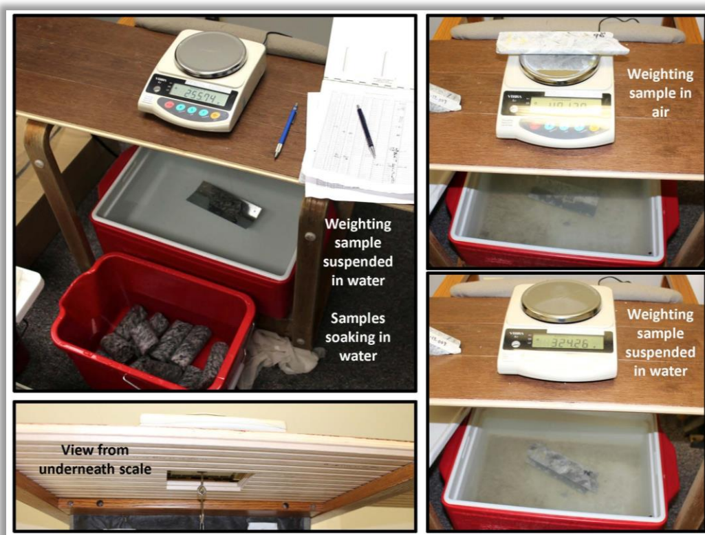
Figure 14.1 Specific Gravity Station
