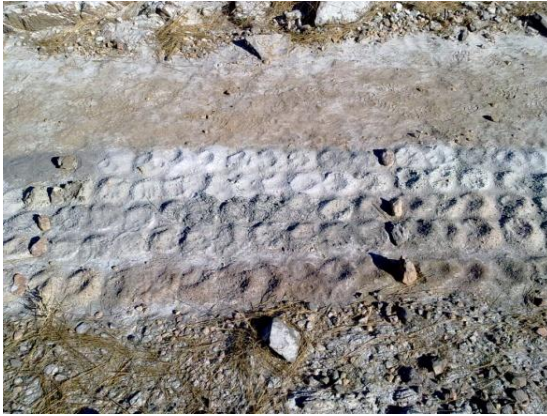
Figure 10.6 Geology chip sample layout and logging (1m intervals).
