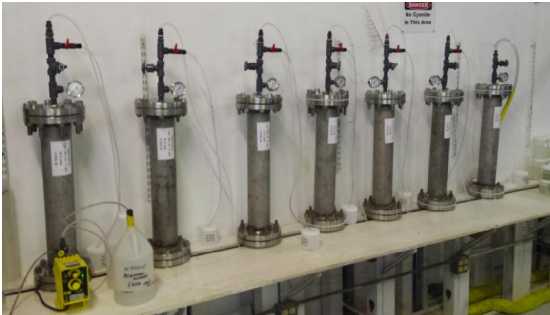
Figure 13-1: Series Leach Test Apparatus
