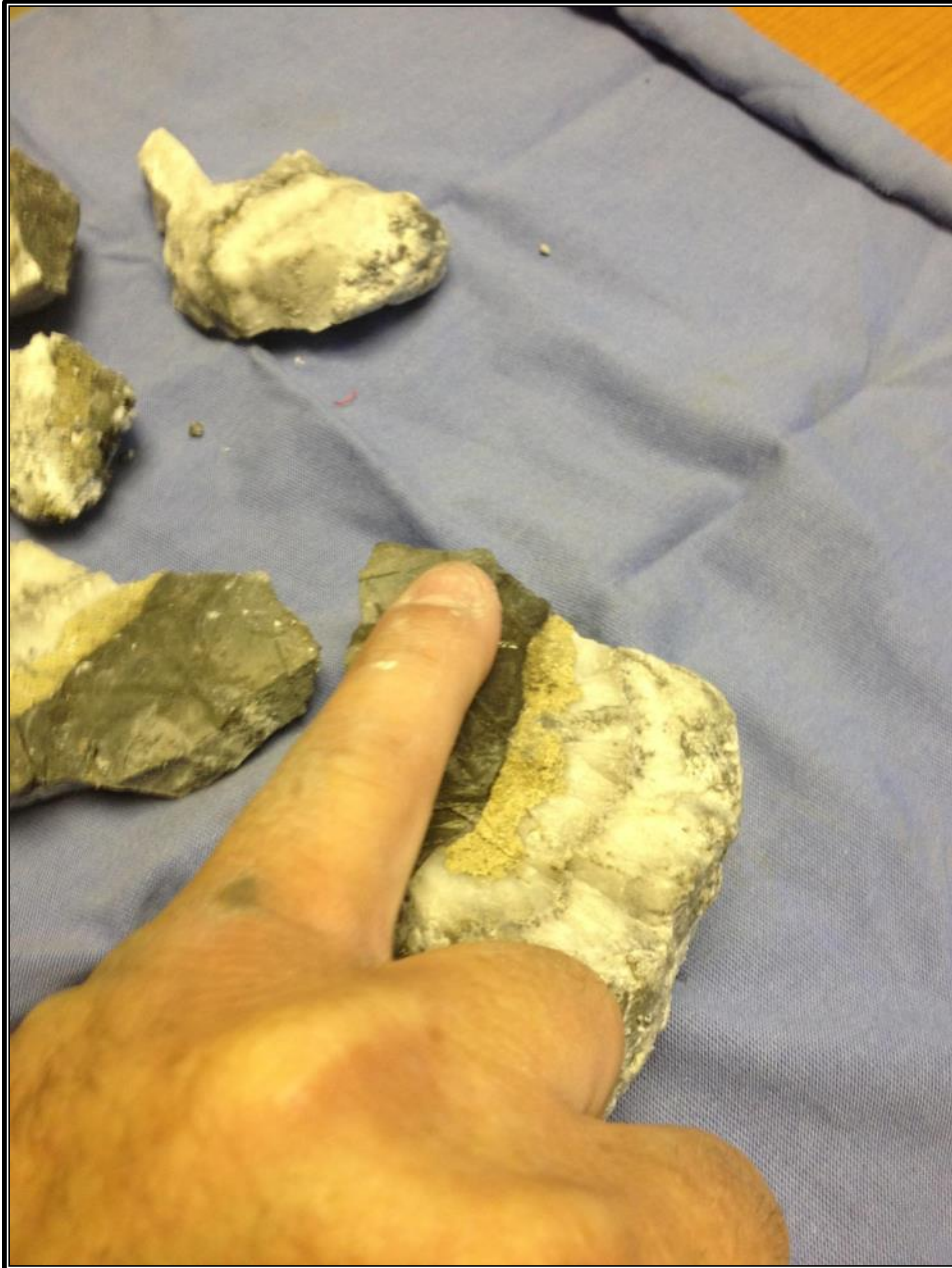
Figure 7-13 Banded Vein Sample from the Vonnie Vein that Contains Large Clots of Electrum Gold
