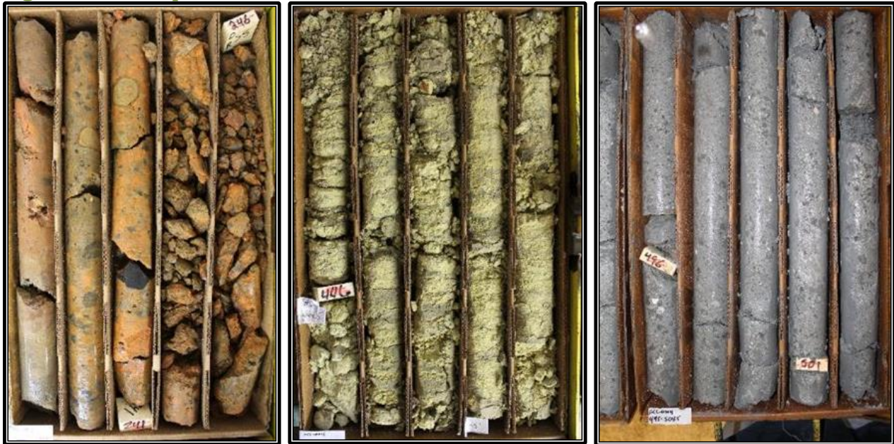
Pictures of whole-core (HQ) with three different examples of Tlat. From left to right: oxidized tuff breccia, oxidized lithic tuff, reduced lithic-lapilli tuff).
