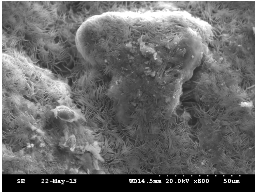
Figure 20.4: SEM image of lab weathered peridotite grains. A smaller peridotite grain is “cemented” to a larger grain through a network of platy carbonate minerals
