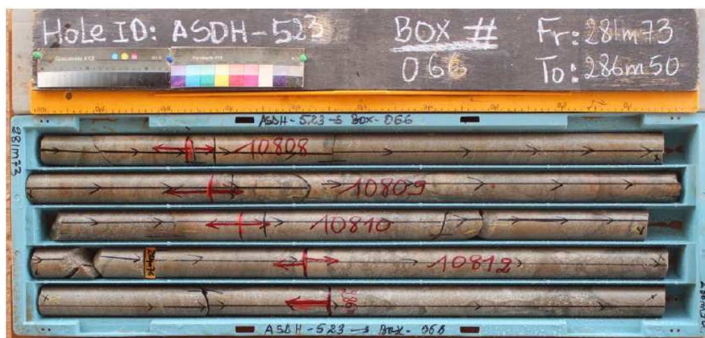
Figure 10-2: Diamond core photograph example
