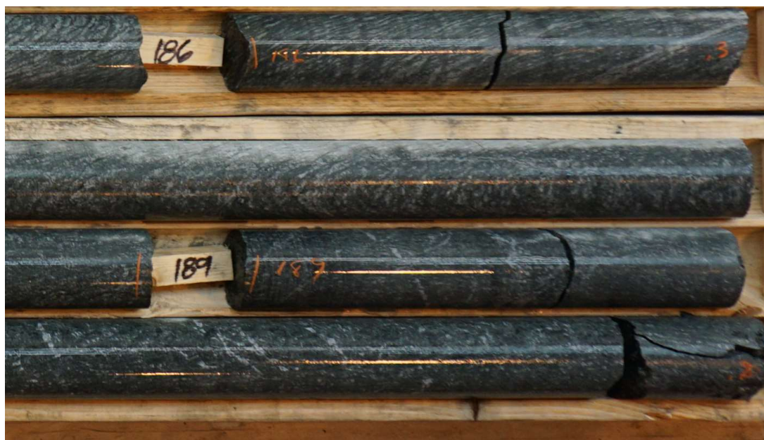
Figure III.8 – Example of chlorite-carbonates hydrothermal zone characterized by the complete disappearance of epidote (Hole CR-15-426)
