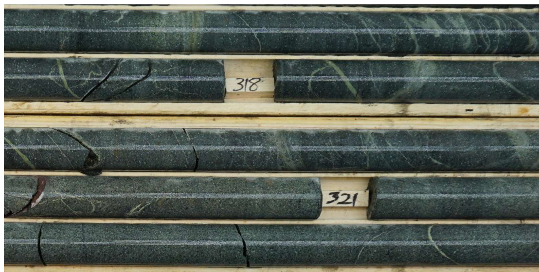
Figure III.7 – Example of epidote-chlorite hydrothermal zone corresponds to the "fresh or unaltered" diorite (Hole CR-15-420B)
