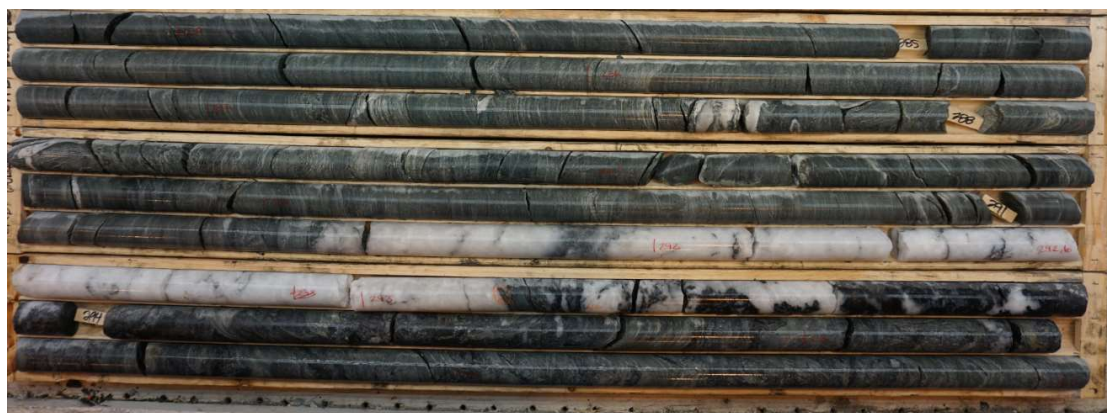
Figure III.1 – Shear vein observed within the hole CR-15-420B
