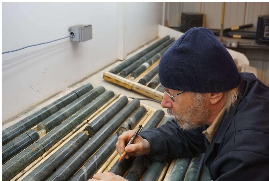
Figure 12.2 – Diamond drill core logging by Monarques geologist
