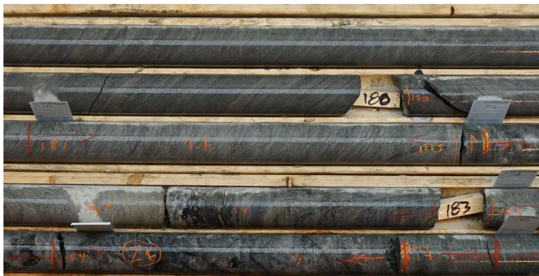
Figure III.9 – Example of sericite-carbonates hydrothermal zone characterized by the gradual and usually complete disappearance of chlorite (Hole CR-15-426)
