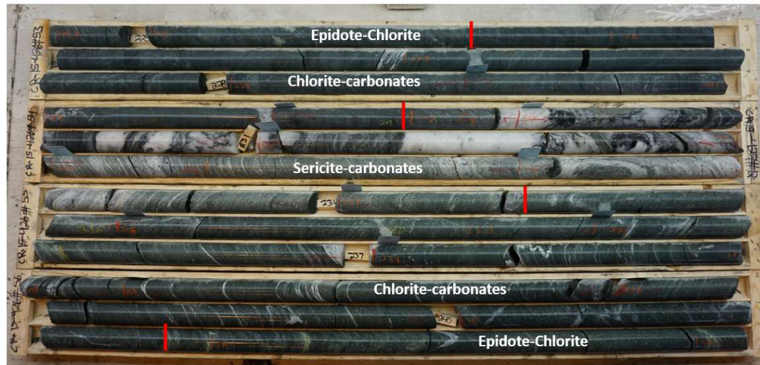
Figure III.5 – Hydrothermal alteration halo surrounds the mineralized zone (Hole CR-15-426)
