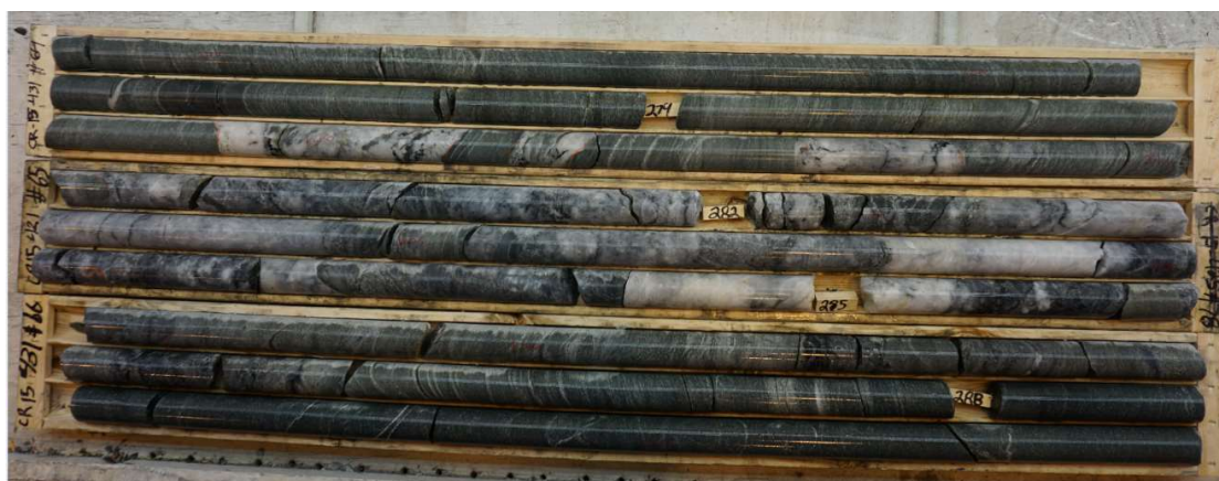
Figure III.2 – Brecciated quartz-tourmaline vein observed within the hole CR-15-431
