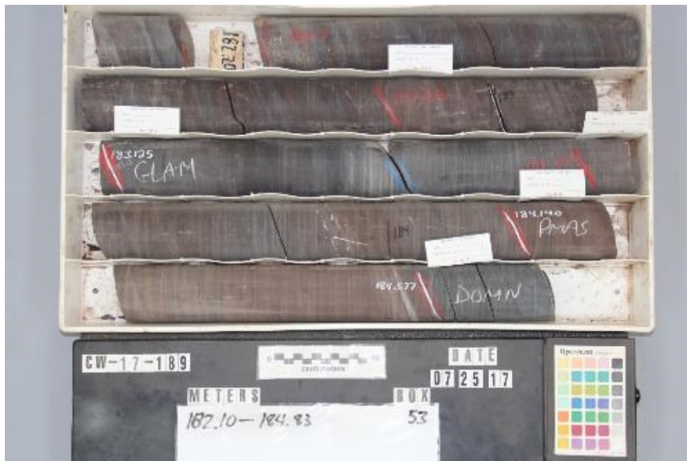
Figure 10.9: Top of LCBS Showing Marked Intervals for Assay Sampling
