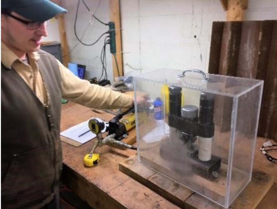
Figure 10.6: Point Load Testing (Bemek Rock tester)
