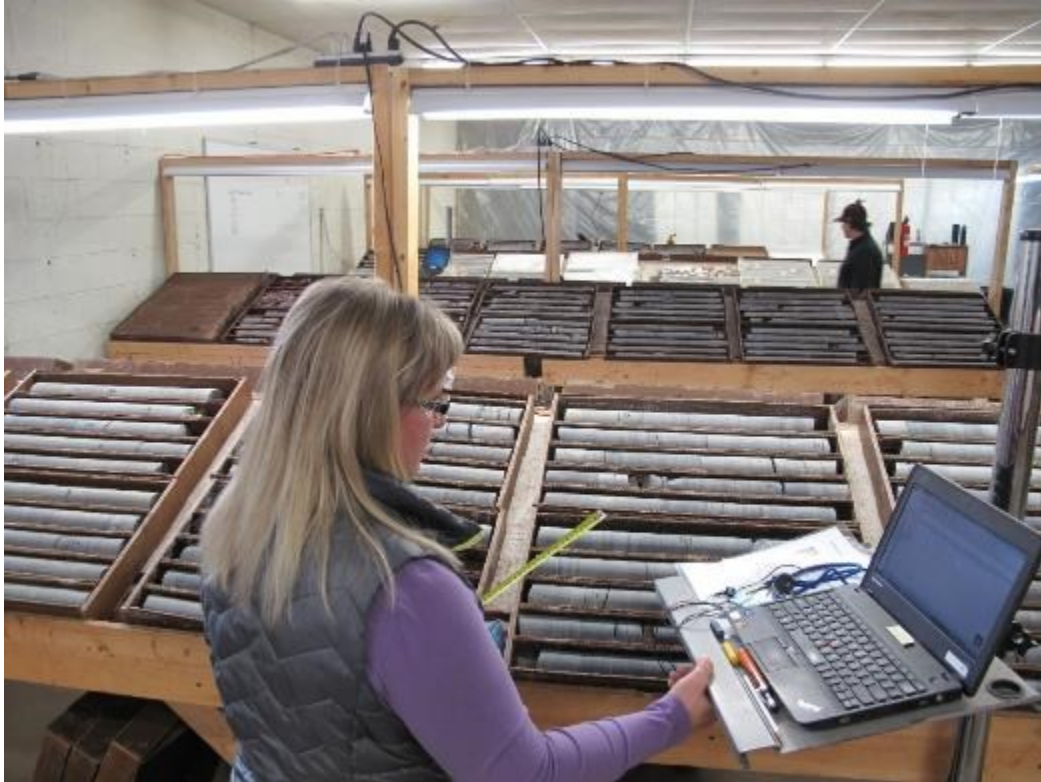
Figure 10.4: Core Logging at White Pine site
