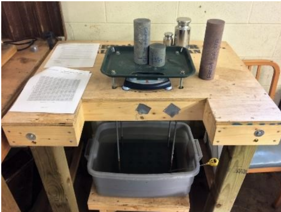
Figure 10.7: Specific Gravity Station
