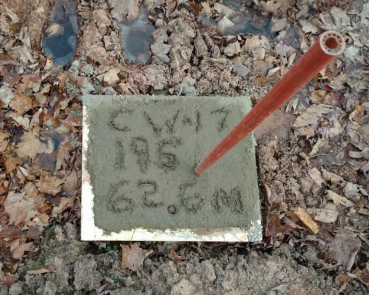
Figure 12.1: Drill Hole Collar Example in Section 6 - CW17-195
