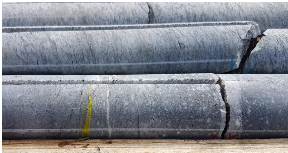
Core orientation line rolled down to groove edge. Cut line in yellow.
