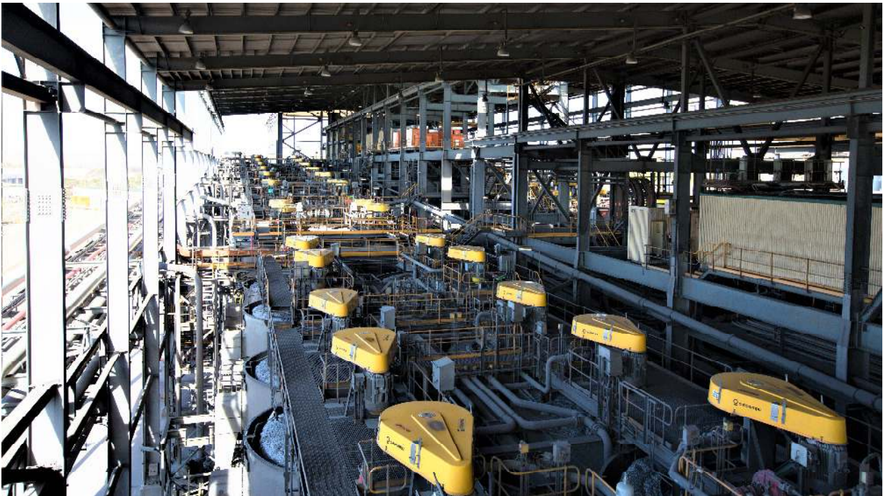
Figure 10: One of two flotation trains within the Century Processing Plant
