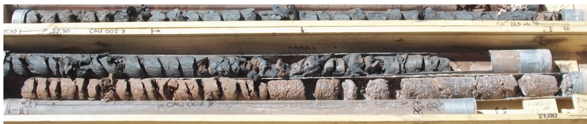
Figure 7.3 Red and black clays representative of Unit A subunits
