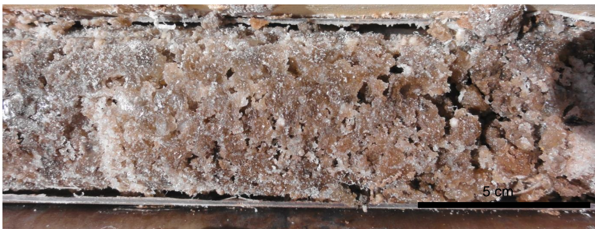
Figure 7.7 Porous halite in unit B2 with possible primary subaerial to shallow water porosity
