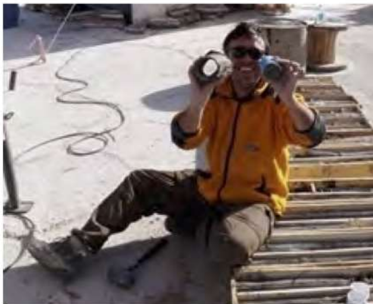
Figure 11.4 Collecting an Undisturbed Sample from Clay Core
