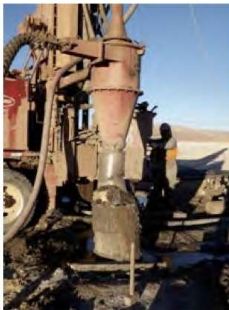
Figure 11.1 Cyclone with Plastic Bag (dry sample)
