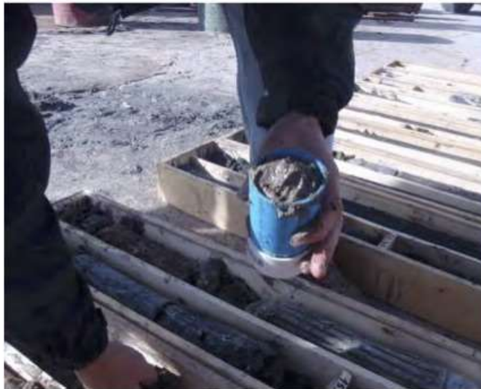
Figure 11.3 Collecting an Undisturbed Sample from Sand Core
