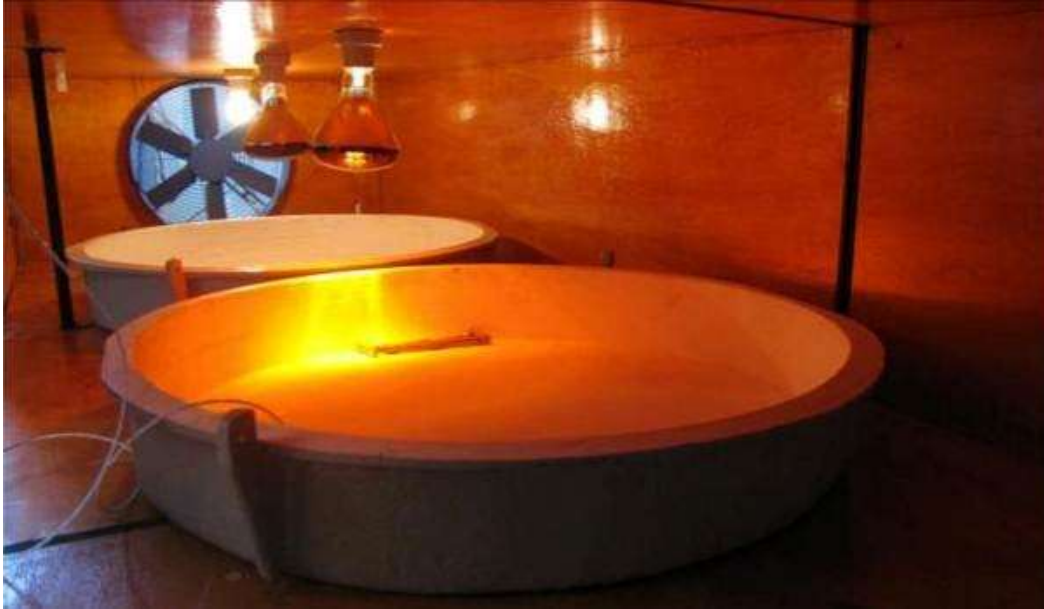
Figure 13.2 Dry Air Evaporation Tests
