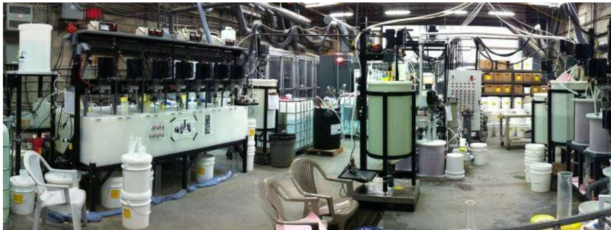
Figure 13.8 Pilot plant (SX-Purification-Carbonation-Filtration-Washing Pulp)
