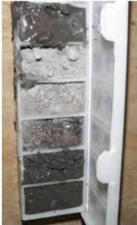
Figure 11.2 Rock Chip Tray with Dry and Wet Samples
