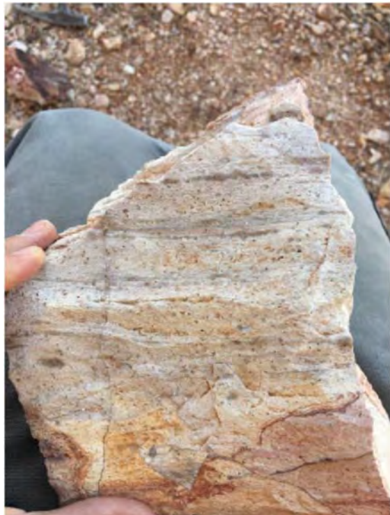
Figure 7-4a – Flow-banded quartz-porphyr rhyolite (QPR), with 1-2 mm quartz phenocrysts in a crystalline groundmass.
