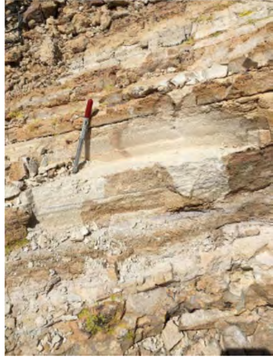
Figure 7-5b – Bedded lithic tuff (LT) with stratified ash matrix and fine-grained lithic clasts <1mm.
