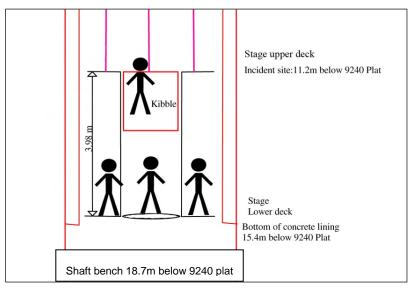
Figure 21. Position of workers in relation to the stage and kibble at time of incident (not to scale).
