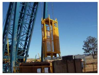
Figure 1. Photograph of a purpose-built man riding cage.
