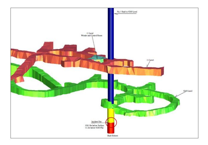
Figure 19. CSA mine plan depicting location of incident site in the No.1 shaft.
