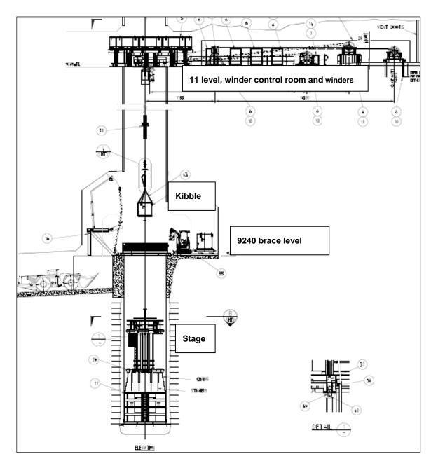
Figure 5. General arrangement plan of the 11 level, 9240 level and shaft sinking infrastructure.
