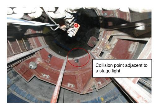
CCTV footage confirmed that the stage lighting was not operating when the incident occurred. The non-operational stage lighting had the capacity to project 480 lux onto the stage work environs. The absence of this lighting created a working environment with limited peripheral illumination and likely impaired situational awareness.
