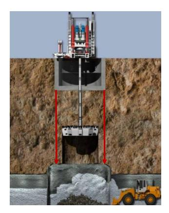
It is important to note that this technique does not involve the use of a kibble and it was intended that the strip and line technique would be undertaken from a single platform shaft sinking stage.
