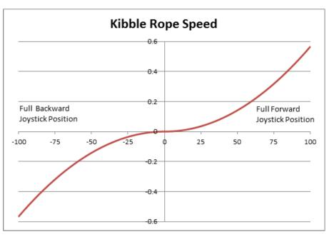
The above diagram highlights that the kibble winder could be operated at any speed up to its maximum speed of 0.55 metres per second. The investigation did not determine the exact speed of the kibble winder when the incident occurred, but shaft workers reported that the kibble speed appeared normal. Subsequent testing of the winder system by investigators found the system to be functional and there was no evidence of winder system error or malfunction.
