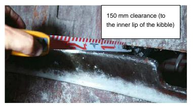
Figure 11. Diagram of ability of kibble well to traverse through the stage.
