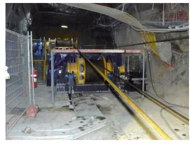
Figure 12. Winders situated on the 11 level.
