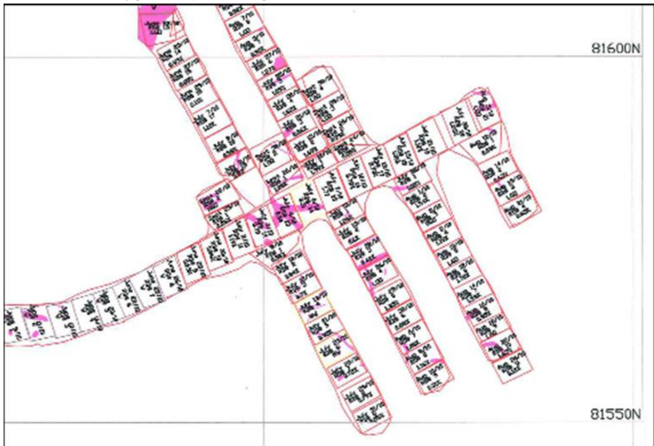
Figure 13: Combined Estimated Geology – Plan View Scoop Nickel Grade Estimates shown within Polygons Representing Drift Round Advance.
