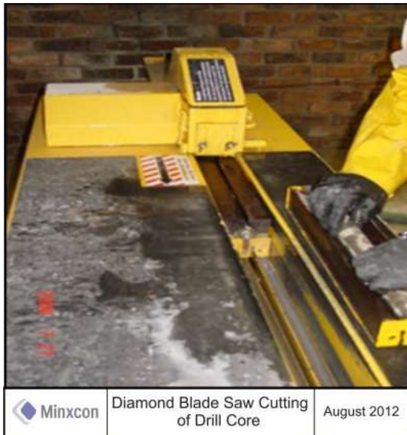
Figure 25: Diamond Blade Saw Cutting of Drill Core
