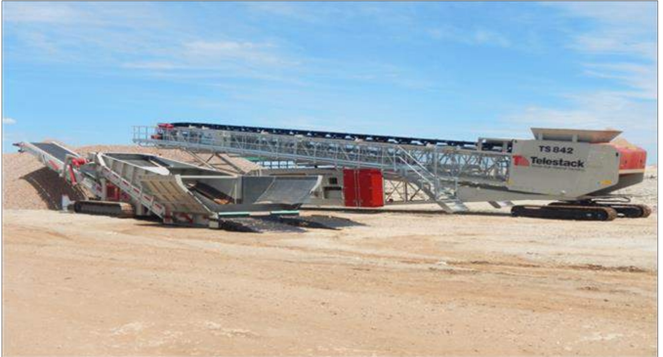
Figure 17-5 Stacker and dump hopper (ready for relocation)
