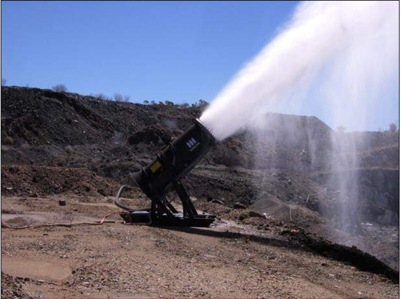
Figure 17-12 Water cannon in operation evaporating water.
