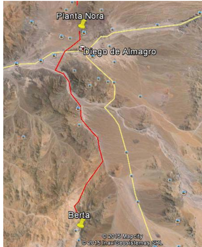
Figure18.2: PLS and Water/Raff pipeline
