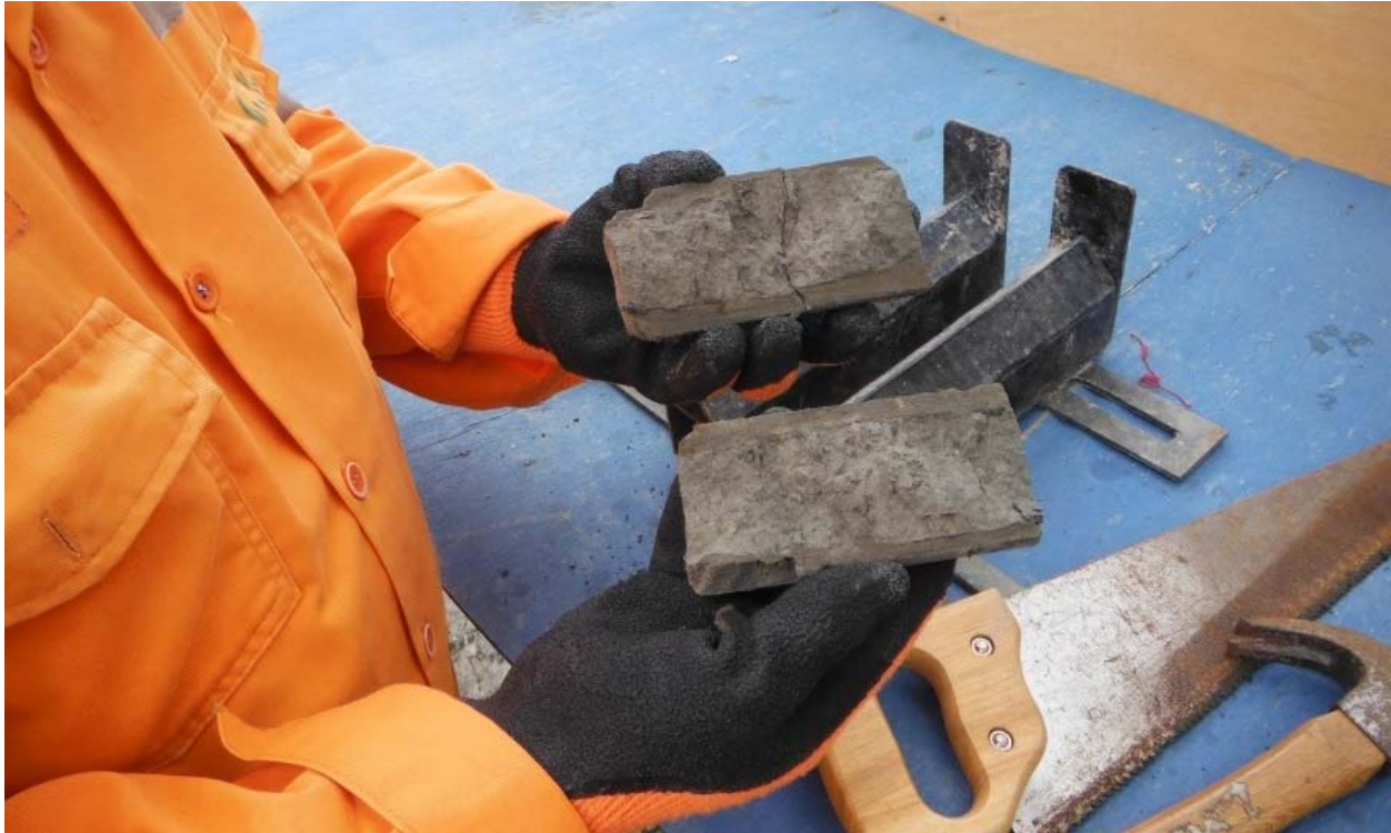
Figure 12-4: Core Splitting Being Performed During the Qualified Person Site Visit
