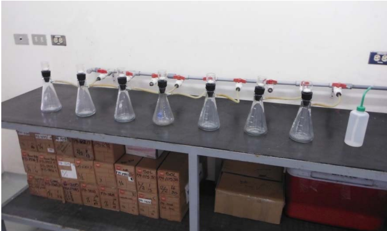
Figure 11-12: Gravimetric Analysis for P_2O_5
