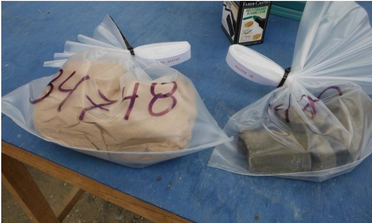
Figure 11-3: Wrapping Phosphorite Sample in Brown Paper to Prevent Sticking in Sample Bag
