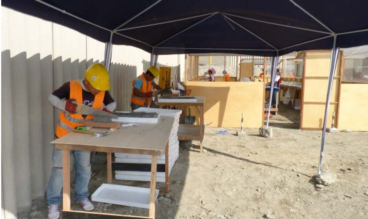
Figure 10-7: Cutting Longitudinal Line on Core Prior to Splitting
