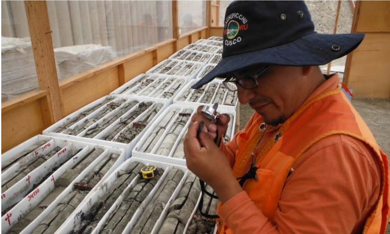
Figure 10-11: Geologist Estimating Pellet Content in Phosphorite and Diatomite Bed
