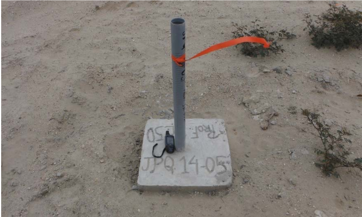
Figure 10-3: Cement monument marking 2014 Bayovar 12 Drill Hole
