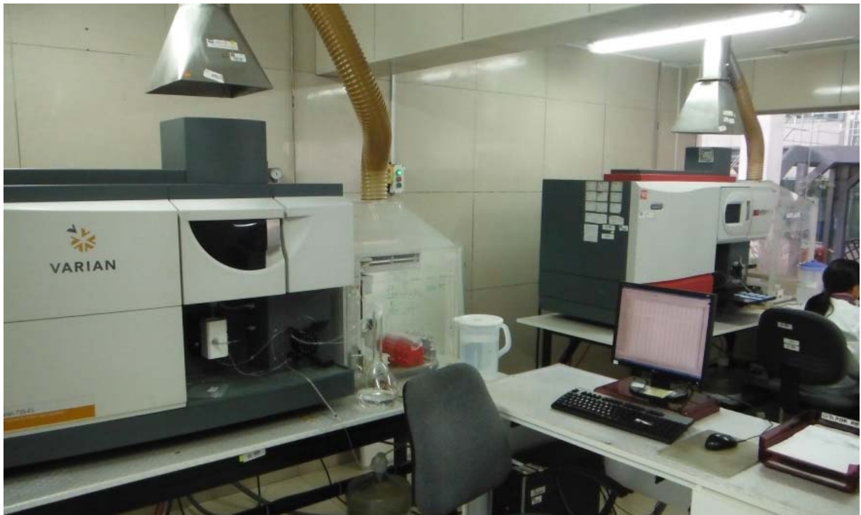
Figure 11-13: ICP-OES analysis for major oxides
