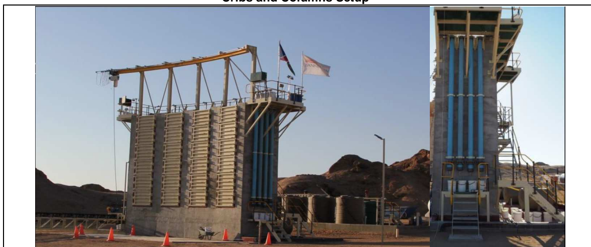
Figure 13.23 Cribs and Columns Setup
