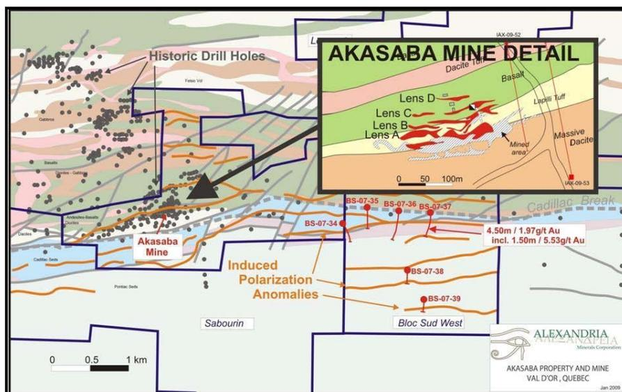
**Figure 6. Schematic interpretation of parallel mineralized lenses identified at the Akasaba mine by Cambior**
